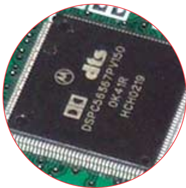
The new DSP chip. Note the Motorola model #56367P
