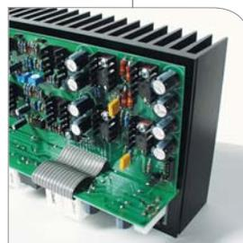
PVA amplifiers can be powered On/Off three ways: manually, with the On/Off switch on the front panel; remotely, via the 12-volt trigger input; or automatically, with our patented Auto-On/Off circuit—an incoming audio signal immediately switches it on, and approximately 20 minutes after the audio signal ends, it simply switches off.
