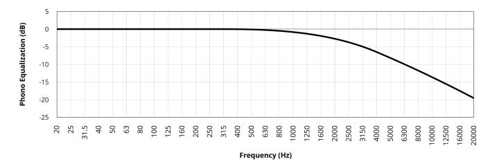
**10K DE-EMPHASIS** – the attenuation at 10 kHz. In this example, it is -13.7 dB:
