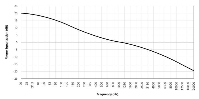
The following curve combines the two above and adds **BASS SHELF** or boost limit at 20 Hz, which is 20 dB in this example:
