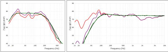
The red curves represent the in-room response before correction, as an average from five measurement positions, whereas the green ones show response with equalization applied. In this case a subwoofer and bass management are also in use. In the subwoofer graph, which is on the left, the difference between the level of the red and purple curves shows the amount of room gain.
